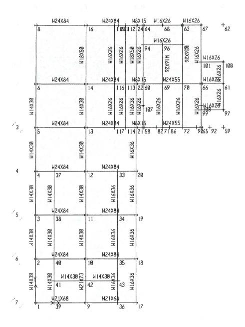
ETABS v9.7.4 - File: LIO-v2.0 - August 28,2013 11:06 Plan View - MAIN ROOF - Elevation 1171 - Kip-in Units
